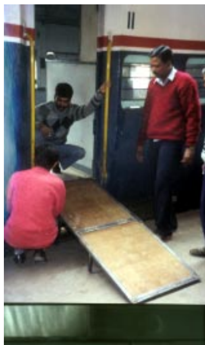
A ramp developed by one of the Voluntary Organisations for use at railway stations.
